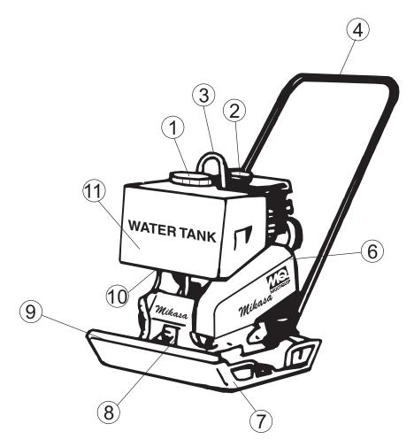
Figure 1. MVC77 Series Plate Compactor Components
